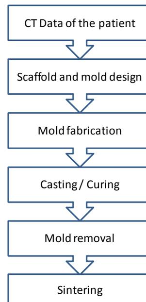
Fig. 1. Schematic chart of the fabrication of customized scaffold via indirect solid freeform procedure.
