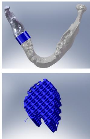
Fig. 3. (a) The jaw bone of the patient with a missing geometry to insure the symmetry like in a healthy jaw bone; (b) CAD modeled a scaffold needed for the treatment.
