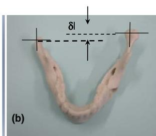
Fig. 2. (a) A typical appearance of the patient having hemifacial microsomia; (b) 3D Model fabricated via rapid prototyping ( $\delta l$ : the missing distance causing the shortness of the bone at one side consequently the distortion on the face)
